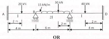
10 Analyze the frame shown in figure using Kani's method.
